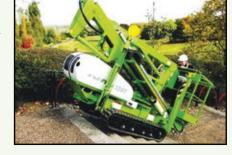
The **TM34T** is also available on low pressure, rough terrain tracks **(TD34T)**.
